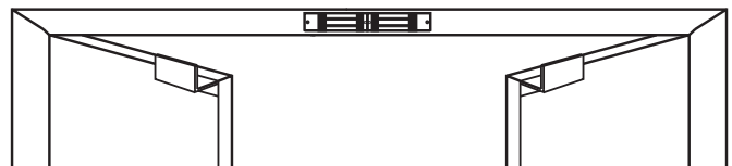
Double Lock, Inswing Door Center Mounted To Header Face With Adjustable Top Jamb "Z" Brackets
