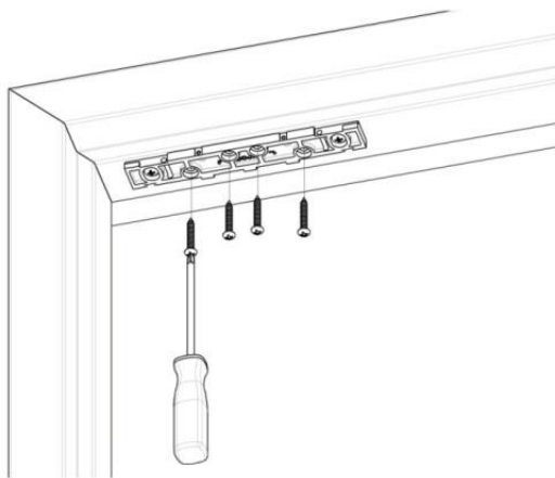
Figure 25. Installing the Anchor Screws
