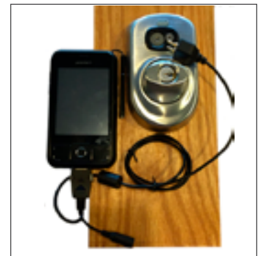
Serial Communication with 2PIN Serial Cable (BM-170)
