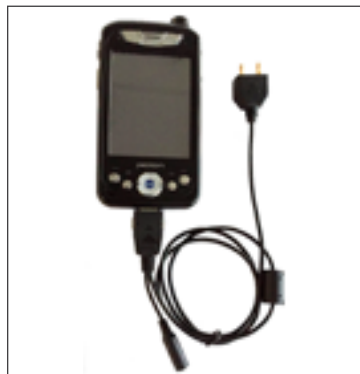
Serial Communication with 2PIN Serial Cable (BM-150)
