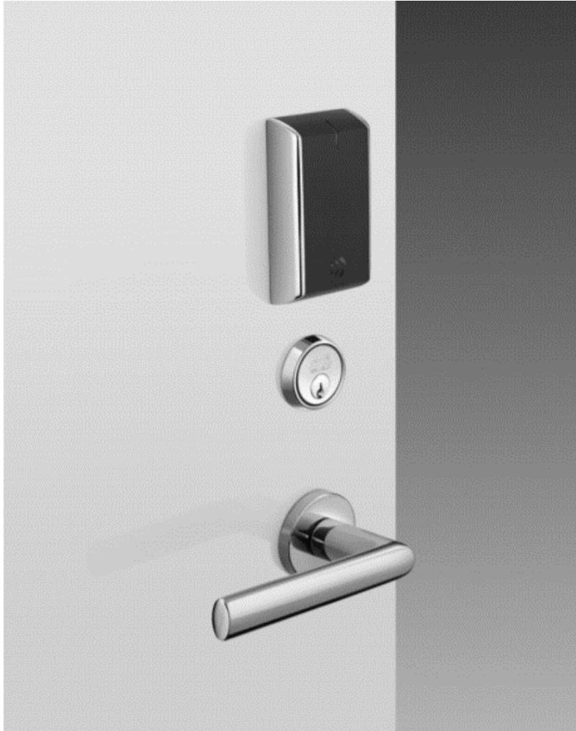
The Corbin Russwin IN120 WiFi mortise lock, is an ANSI/BHMA A156.13 Series 1000 Grade 1 mechanical mortise lock. It has a reversible stainless steel latch, independent non-handed stainless steel deadlatch. The IN120 is an intelligent WiFi Access control mortise lock with integrated credential reader.
